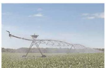
To illustrate how demand charge can affect your bill, let's look at a few examples: We will use a 50 hp irrigator well pump that uses 37 kW with a pivot that uses 3 kW. Combined, the system will have a demand of 40 kW.
